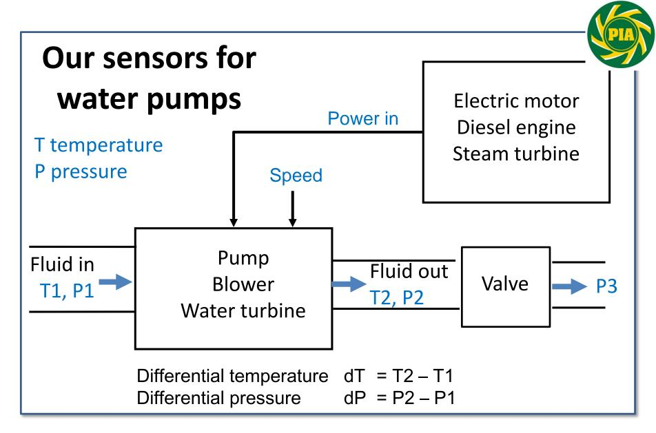
Water is compressed in the pump and has a higher internal energy per unit mass at discharge (T2 > T1 ; P2 > P1)
